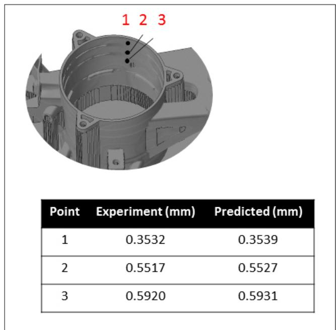
Figure 3 B: Comparison between experimental and predicted distortion
