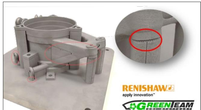
Figure 1 A: Printed wheel carrier. Separation observed in the support structure
