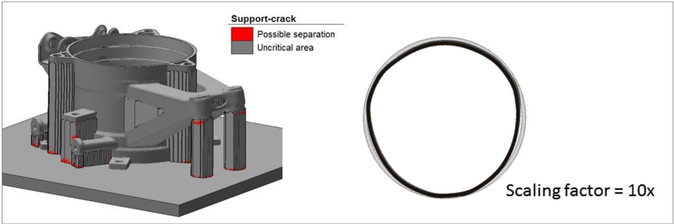
Figure 4: Simulation results with calibrated inherent strains. A- fracture areas, B- Shape of the part with scaling factor 10x
