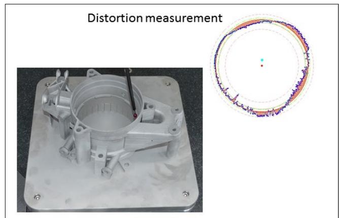
Figure 1 B: Measurement of the distortion at the top of the part
