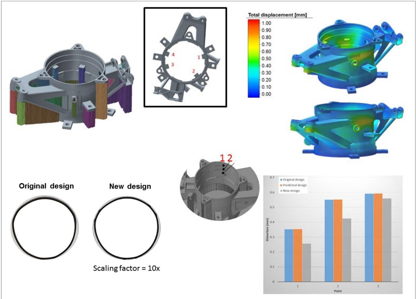
Figure 5: Simulation results of optimized part. A- New design, B- Distortion, C- Shape of the part with scaling factor 10x, D- Comparison of distortion values
