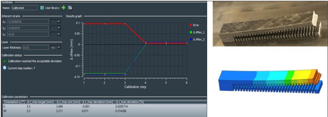
Figure 2: Calibration of inherent strains
