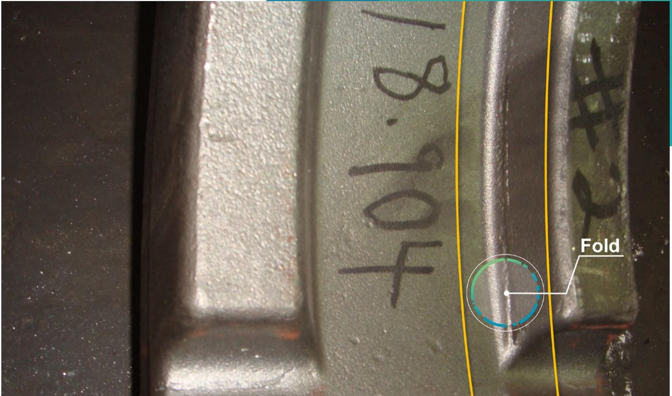
Figure 1: A fold occurred during the production of a forging that had to be rejected
