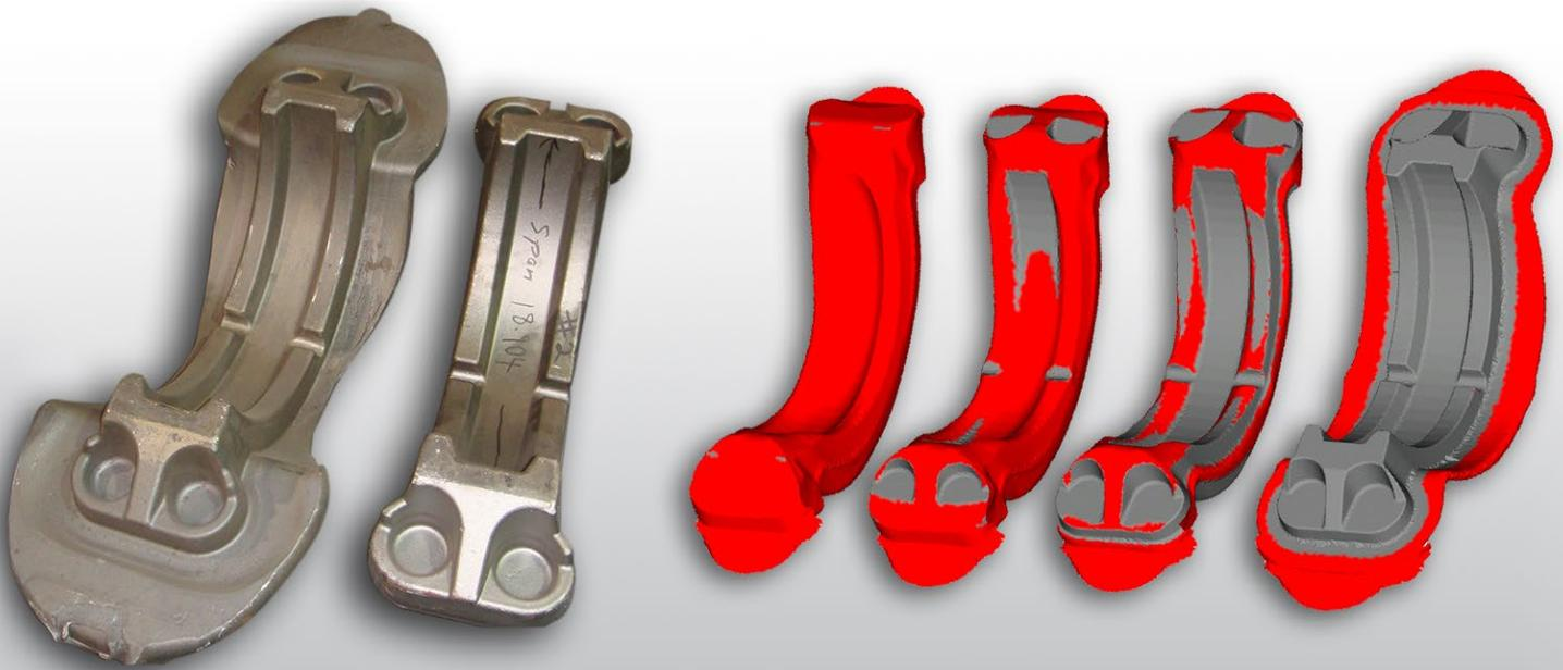
**Demshe Forge Inc. uses Simufact Forming to develop tooling and process parameters for hot forging processes of large parts manufactured with hammer presses.**
