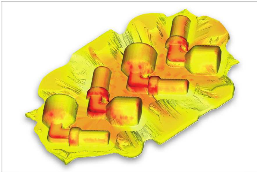
Temperature Profile for the Quadruple Forging of a Brass Elbow
